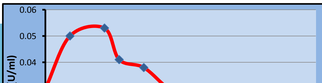
Figure (4-27): Gel filtration chromatography for AmpC \beta -lactamase extracted from PABL positive Klebsiella pneumoniae K19 isolate, using sephadex G75 column with dimensions (1.5 x 45 cm), column equilibrated by 0.05M sodium phosphate buffer (pH 7.0) at a flow rate of 12 ml/hr the eluted fractionated size was 3 ml for each fraction.
